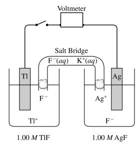
It is observed that when silver metal is placed in aqueous thallium(I) fluoride, TlF, no reaction occurs. When the switch is closed in the cell represented above, the voltage reading is +1.14 V.
